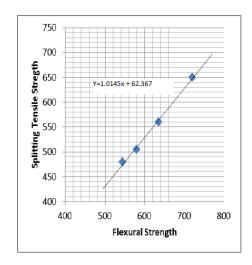
Using this example plot, a contractor's flexural strength result from a set of beams is below 570 psi and chooses to core the pavement to replace the low flexural strength results. If the splitting tensile results from the cores is 535 psi the corresponding flexural strength would be 605 psi. Since the core flexural strength is greater than the cast beam flexural strength, the core flexural strength will be used for determining the incentive/disincentive in SMM.
